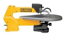
The Scroll Saw is used to make intricate cuts in wood up to <sup>3</sup>/<sub>4</sub> inches thick. The saw blade moves up and down and cuts on the down stroke. To avoid accidents, the following operational safety rules must be observed by everyone working on the GWG Scroll Saw. Failure to be certified or to follow the safety rules will result in loss of shop privileges.
